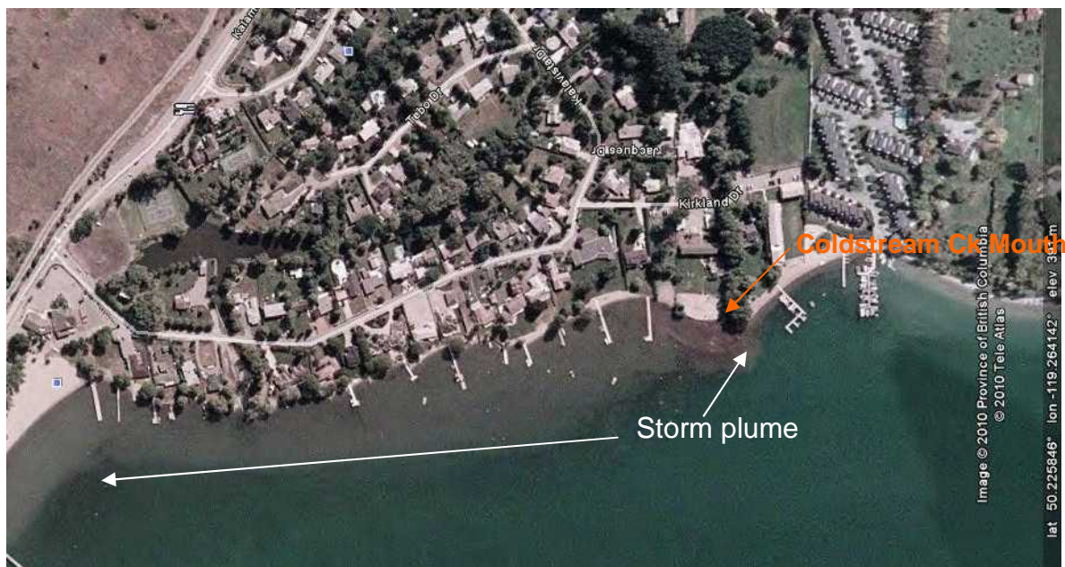
Figure 3.2 Coldstream Creek Storm Plume Deflecting NW Toward Public Beach
